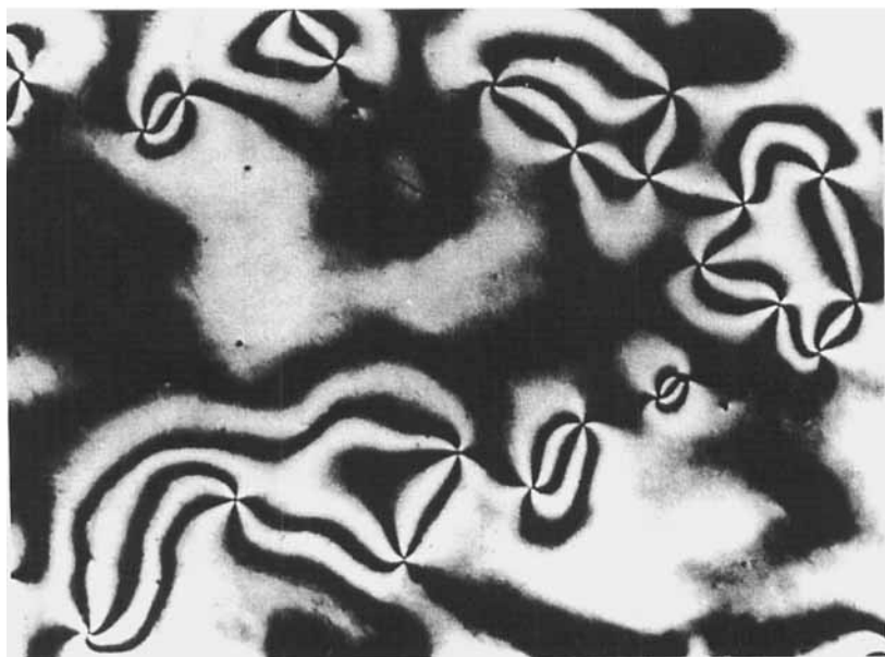
FIGURE 11 Substance No. 7. Smectic F, schlieren texture, 107°C, \times 250 .
