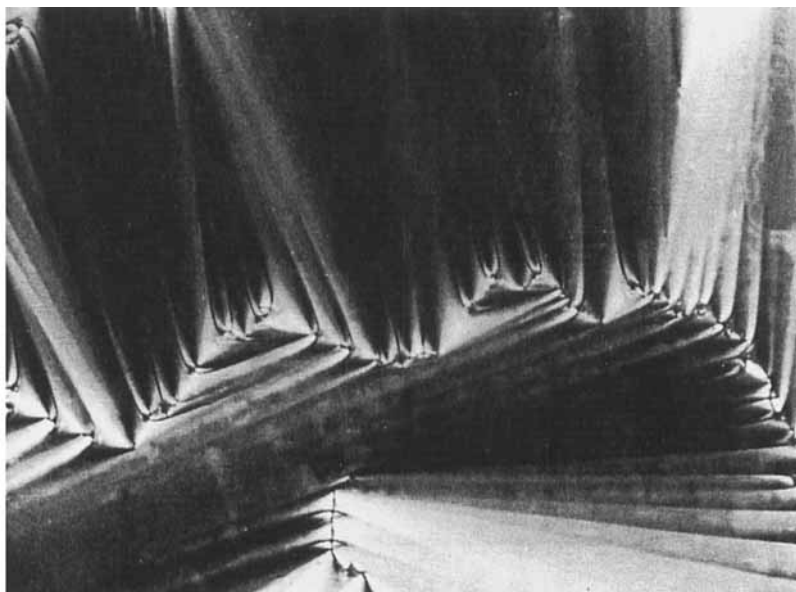
FIGURE 4 Substance No. 7. Smectic A, fan-shaped texture, 150°C, \times 250 .
